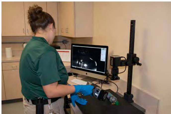
The program runs in live time to help the operator visualize prints and photograph them in one step.
