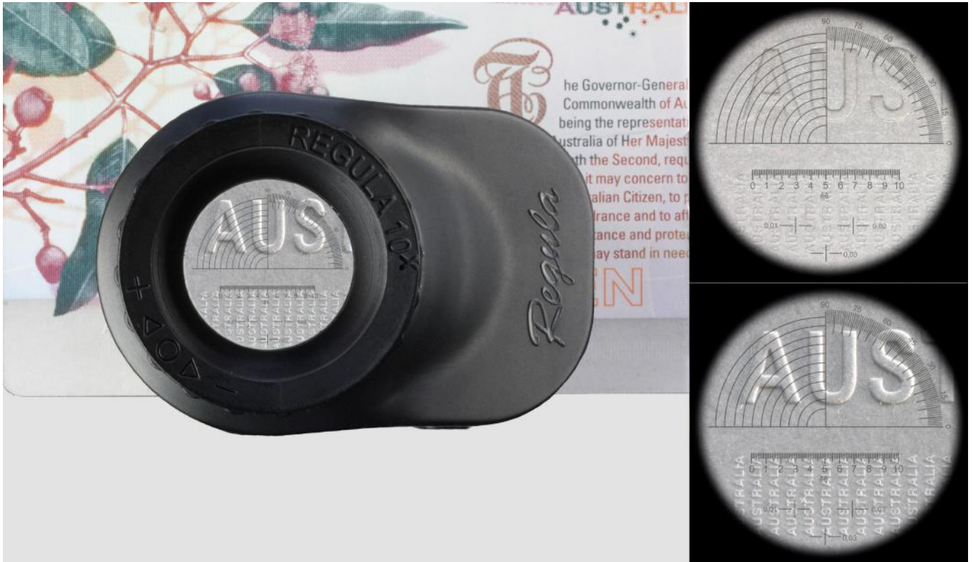
Regula 1004M on a passport page - LED light sources: incident white, oblique white - 10x magnification
