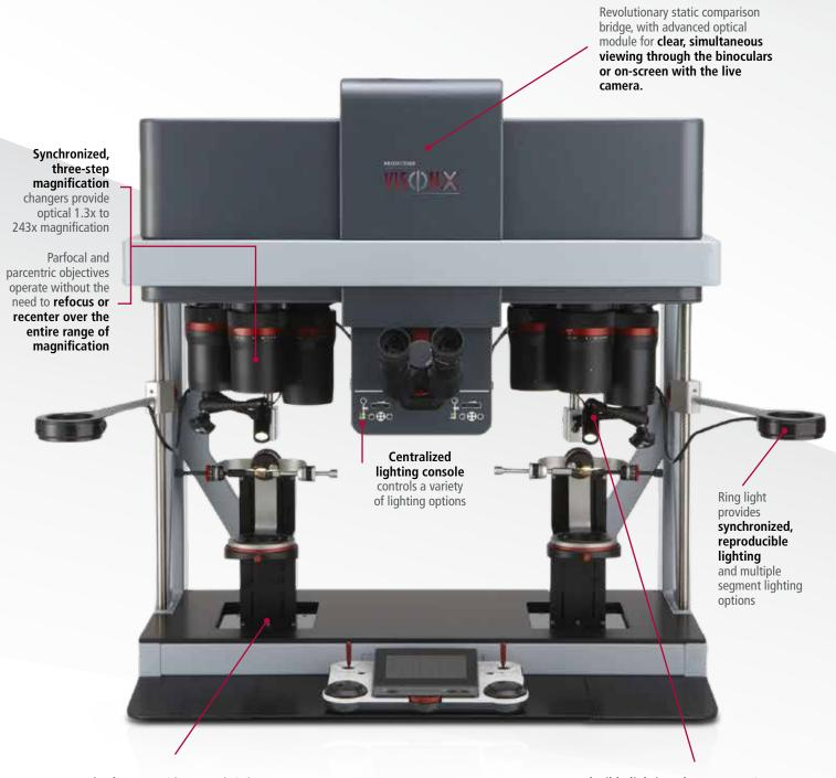
**Motorized stages** with 50 mm (2 in.) of X/Y movement and a height adjustment of up to 146 mm (5.8 in.)
